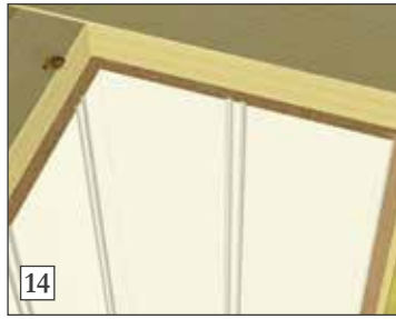
14) Make sure the panel is completely knocked in.
