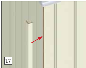
17) At external corners use the Huntonit corner profile
