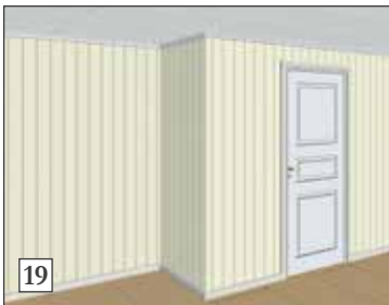
19) This provides a perfect external corner. The external corner profile may also be glued on.
